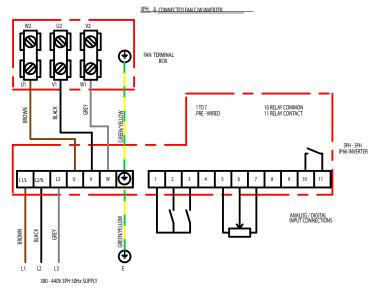
All wiring and control equipment must comply to the latest IEE regulations, in particular part 552-01-02/03. MK-152-617 Issue B: 10.09.2018
